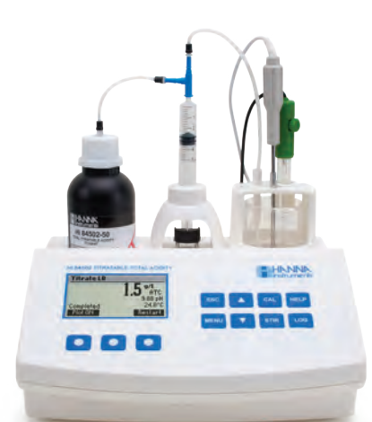
HI84502 Total Acidity Mini Titrator and pH Meter for Wine Analysis Reagents and Accessories
